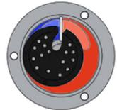
5- At the end of the cycle, the inlet measuring chamber takes all the space. From this moment it can be considered that this is already the outlet chamber, so we are again at the beginning of the cycle.
