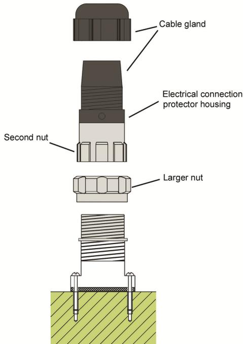
Loosening the larger nut in the middle of the connector allows us to withdraw the half where the cable will be later soldered.
