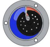
3- The liquid fills progressively the inlet measuring chamber (in red), as it is getting emptied on the outlet (in blue). In the middle of the cycle (see figure) the two chambers are the same size.
