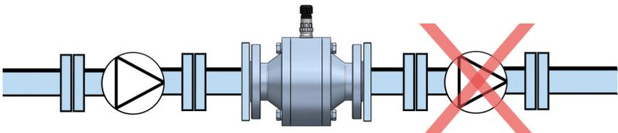
This way the presence of air pockets in the flowmeter is avoided, which could cause false readings. In particular, the associated electronics would show a volume higher than real.
