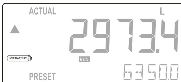
Fig. 6: Example of low-battery alarm.
