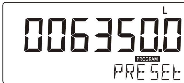
Fig. 3: Example display information during programming preset value.
