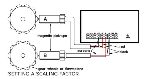
When power is first applied to the instrument it will be in the RUN mode. In order to engage the SET mode remove the bezel and front cover to reveal the switches. Hold switch 'A' depressed and press switch 'B' once. On releasing switch 'A' the display will show SET for one second followed by the scaling factor contained in the memory. The L.S.D. will now flash and the scaling factor can be set using switch 'B' to set the value of each digit and switch 'A' to select the digit.
