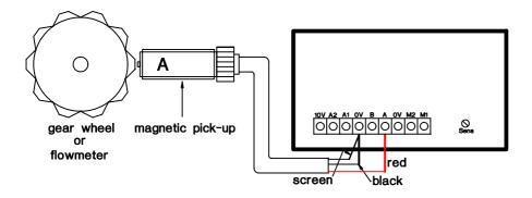
If the display reads '-SIG' it indicates that no signal is connected. Should the instrument still read '-SIG' when a signal is applied then the sensitivity must be increased by adjusting the control in a clockwise direction.
