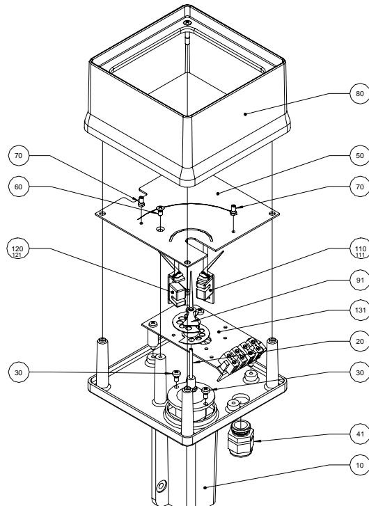
**16.2.4 Complete indicator unit with E2 KINAX Ex transmitter**
