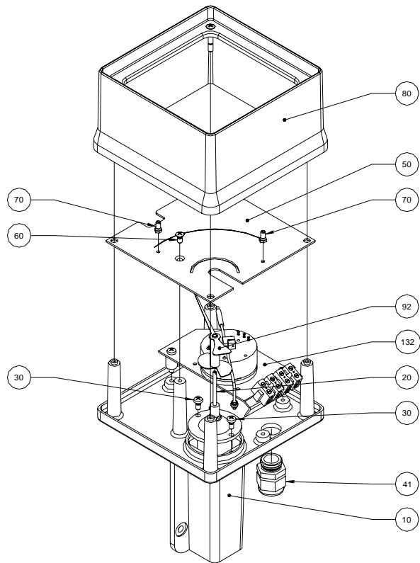
**16.2.5 Complete indicator unit with E2 KINAX Ex transmitter and 1 SJ 3,5 N limit transducer**
