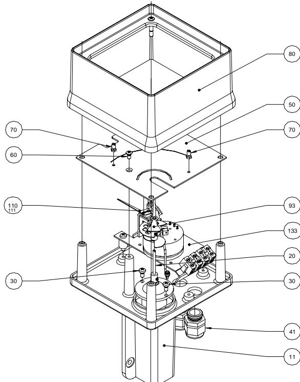
**16.2.6 Indicator unit with transmitter type ES Ex HART®**
