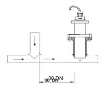
Control valves or stop cocks should always be installed downstream from the sensor to assure that the pipe is always full of liquid.
