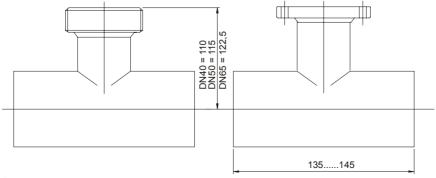
For DN greater than 65 mm for each of the two types of fittings there are three lengths.
