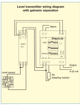
The adapting resistor value should be ten times the resistance of the level sensor at minimum level. Normally the level sensors have a resistance of 1000 ohms/meter and a 2,5 meter long level sensor would have an adapting resistor of  $25k\Omega$ . On demand communication with HART, Profibus of Fieldbus protocol.
